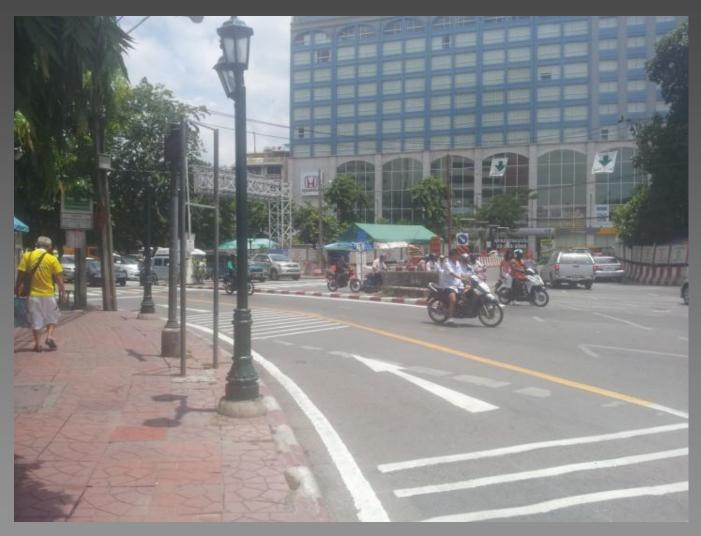
Driver's approach to crossing southbound, incorporating directional arrows and yellow lining making clear traffic flow. 'Rumble' strips emphasising the need to SLOW.
