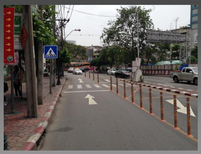
The combination of white directional arrows, coning and removing the old 'STOP' line marking in lane 5, together with installing prominent vertical signing at the crossing, would make the road geography clear to both pedestrians and drivers.
